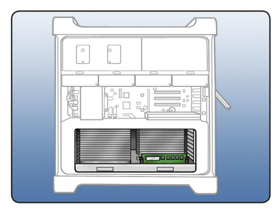
11 Press down and release 2 latches on front of processor tray.
